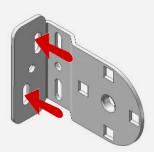
Holding the fully-wound blind, insert the idle pin end into the bracket as shown.
