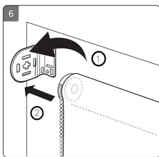
To install, hold fully wound roller against the pin bracket 5 so the pin is depressed. Follow with the opposite control mechanism, raise slightly above the bracket and lower to click into position.
